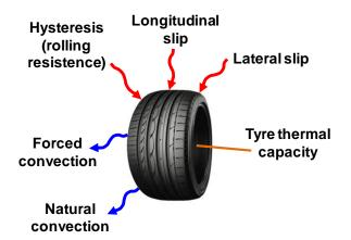
The model takes as input the vehicle dynamic signals (e.g. accelerations, vehicle speed, etc.) and returns as output the tyres internal and tread temperatures based on energy balances.
